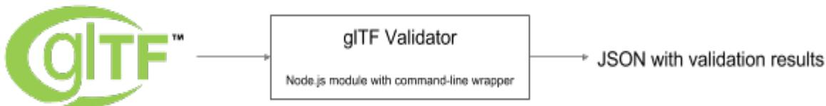
1. Create Validator Tool/library to verify that an asset conforms to the glTF specification, including the simple rules enforced by the schema and the more involved rules detailed in the specification. The entire specification must be supported including separate and embedded resources, geometry, materials/textures/shaders, animations, skins, and cameras. Validation will be divided into four areas:
