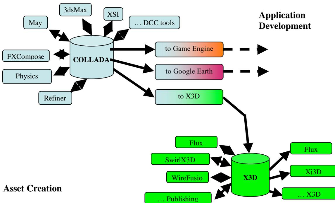
Figure 2. A Typical Web Pipeline Using COLLADA and X3D
